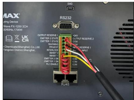
Controller PLC Socket
