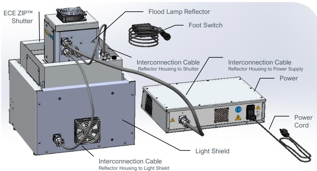
**WARNING!** Do not position the Light Shield on top of the Power Supply (Figure 4). The ECE Flood Lamp System requires adequate air circulation. Setting up the system in such a configuration can result in damage to the equipment and unsafe operating conditions.
