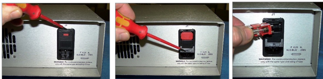
Figure 10. Replacing Fuses in the Power Supply
