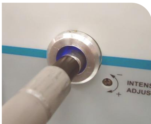
Figure 6. Insert Lightguide into Lightguide Mount
