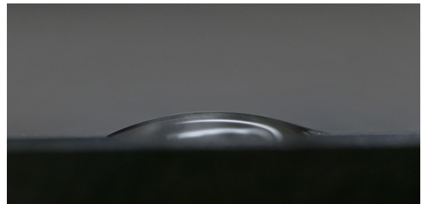
Figure 4. High-energy surface (liquid spreads out, indicating good adhesion)
