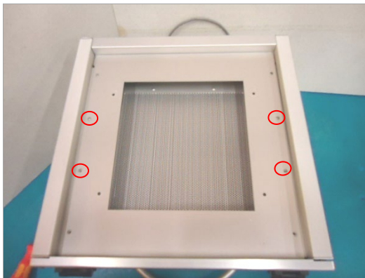
Figure 7. Remove Screws from Light Shield Top Cover
