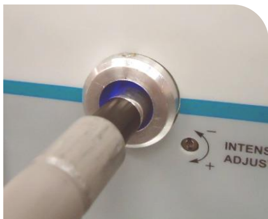
Figure 6. Insert Lightguide into Lightguide Mount
