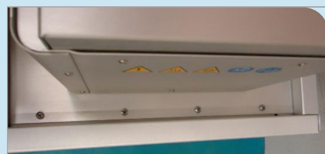
Figure 5. Connect the Lamp/Top Cover Assembly to the Light Shield by reinstalling the eight M4 x 8 mm Screws
