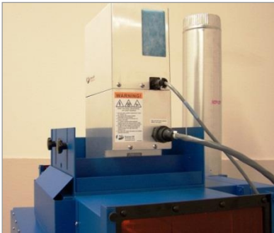
Figure 21. Connect Irradiator Cables to Irradiator (1)
