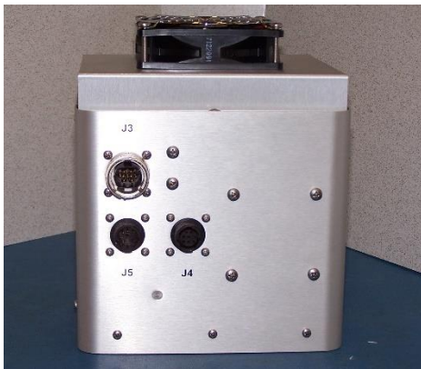
Figure 6. Reflector Receptacles (Rear)
