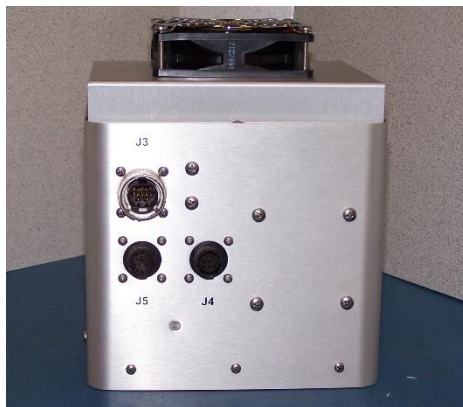
Figure 6. Reflector Receptacles (Rear)
