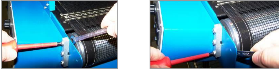
Figure 33. Loosening Drive-Roller Shaft-Support Fasteners
