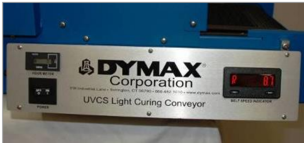
Figure 15. Conveyor Front Panel
