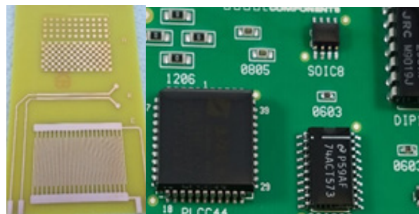
Figure 4. Multi-pattern FR4 test coupon and populated test board
