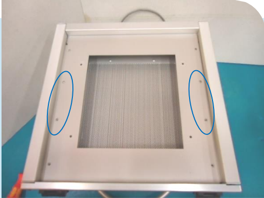
Figure 4. Remove Screws from Light Shield
