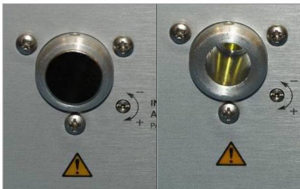
Figure 4. Lightguide Mount Protective Cover Installed (left); Protective Cover Removed (right)
