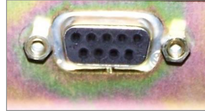
Figure 13. 9-Pin I/O Signals
