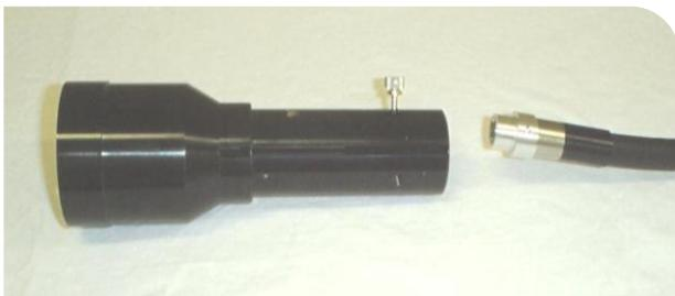
2. Place the adapter on the end of the 8-mm lightguide & gently tighten the setscrew.
