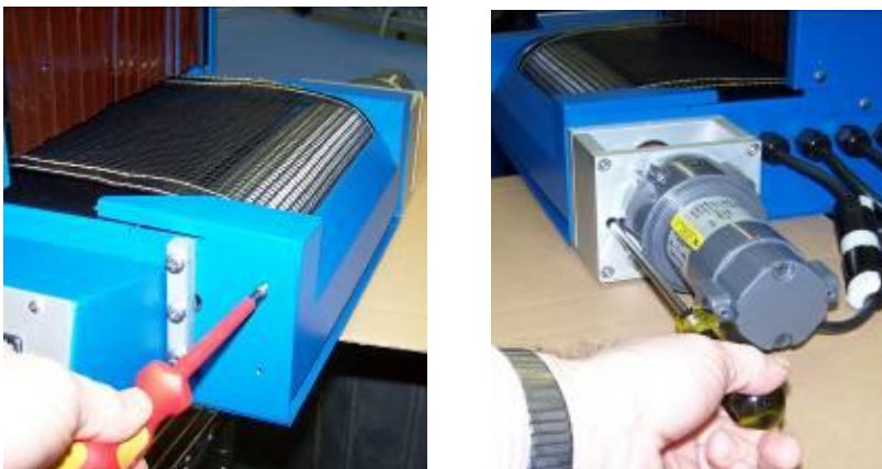
Figure 22. Installing Pinch Guard (front & back)
