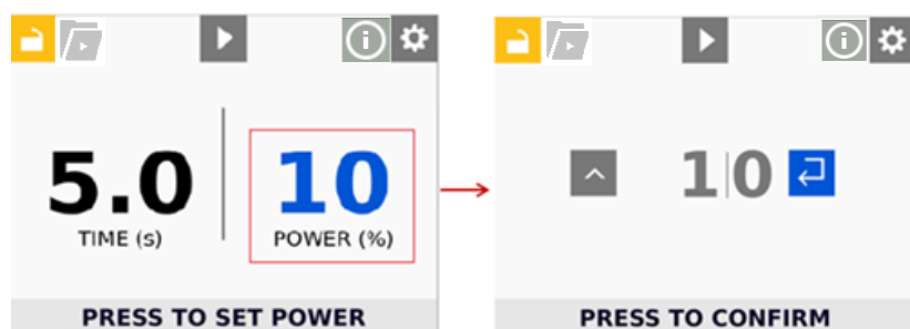
Figure 40. Power Level Screen
