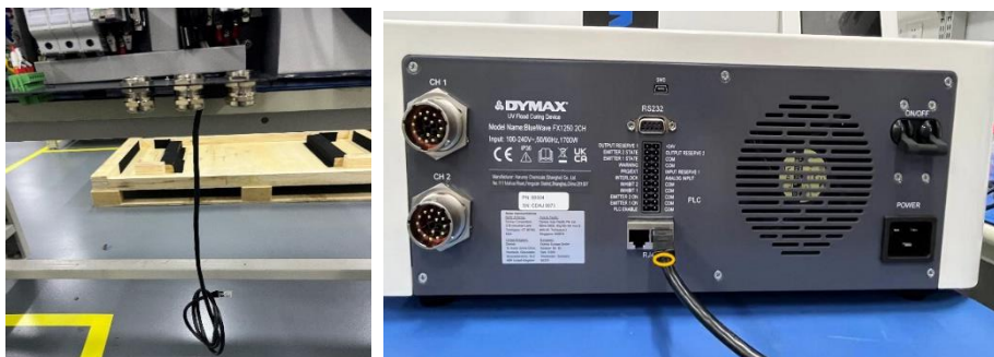
Figure 34. Plugging Connection Cable into Controller
