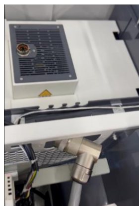
Figure 24 Cable Connector goes through the Wire Slot
