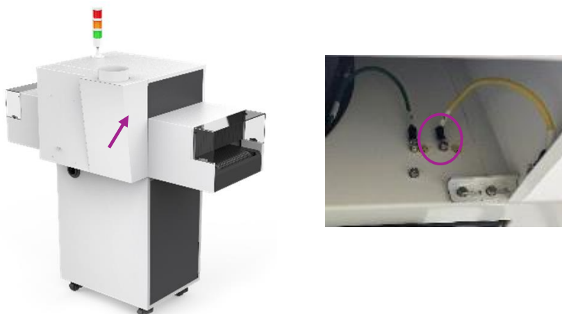
Figure 14. Remove the Grounding Wire inside the Back Panel at the Position as Shown
