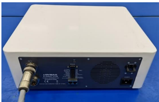
Figure 34. Plugging Connection Cable into Controller
