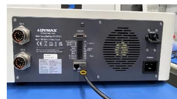
Install Connector and Network Wire on the Controller Connection
