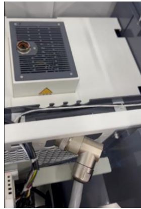
Figure 24. Cable Connector goes through the Wire Slot
