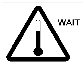
Figure 29. LED Head Has Overheated
