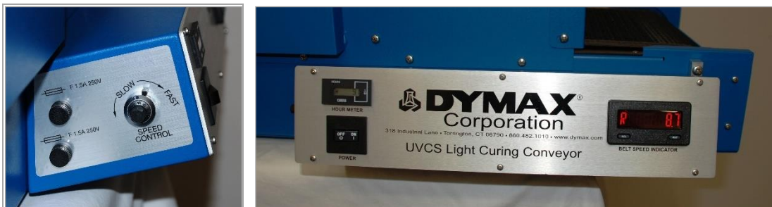
Figure 6. Conveyor Control Panel
