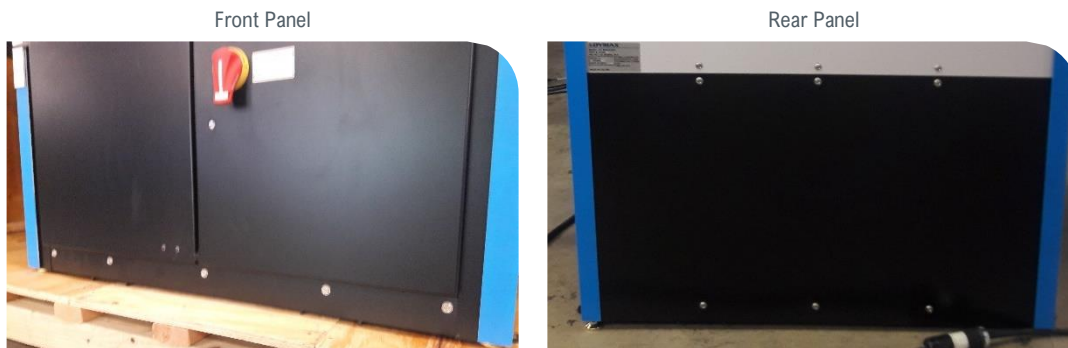
Figure 1. Front and Rear Panels - Remove for Forklift Access
