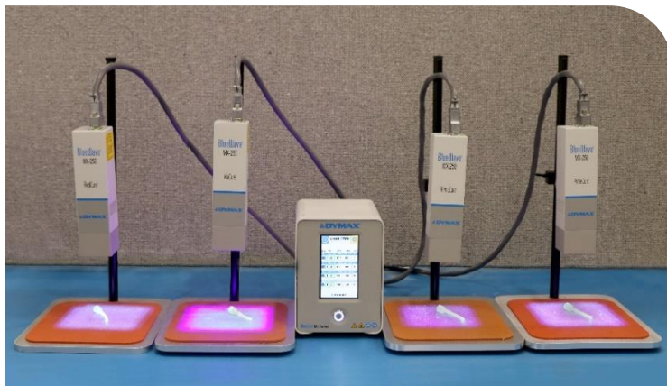
Figure 2. BlueWave® MX-250 System with 4-Channel Controller
