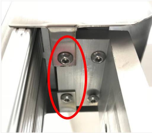
Figure 2. Remove 2 Mounting Screws
