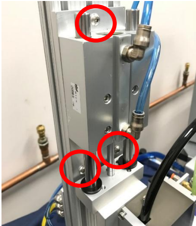
Figure 4. Loosen 3 Bolts on Cylinder Mount Adapter
