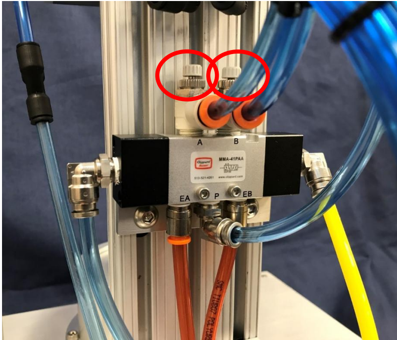
Figure 10. Operating Valve and Flow Controls
