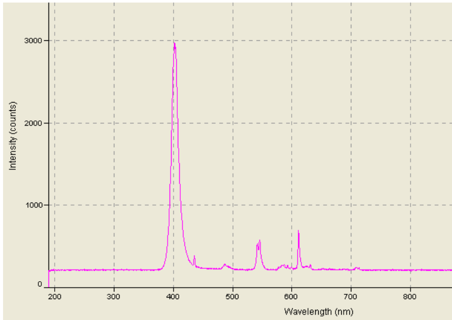
Figure 18. BlueWave LED DX-1000 Spectral Output
