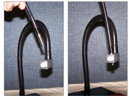
Figure 2. Insert Lightguide into Lightguide Holder
