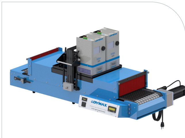
Two Emitters, Mounted Side-by-Side, 10" Wide Single Exposure
