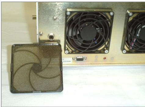
Figure 13. Exhaust Fans with Fan Filters Removed
