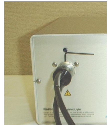
Figure 6. Insert Lightguide into Lightguide Mount
