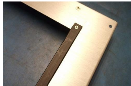
Figure 35. Install M3 x 6 mm Screws into Wear Strip
