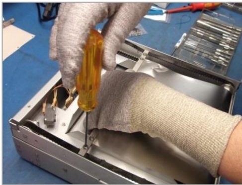
Figure 30. Tighten the M4 x 6 mm End Screws
