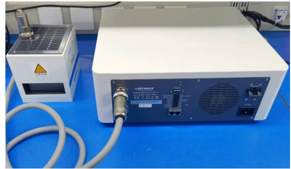
Figure 7. Interconnect Cable Installed
