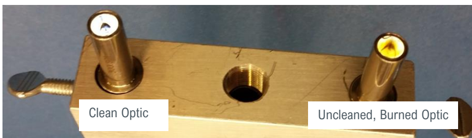
Figure 4. Damaged, Burned Lens
