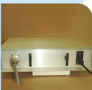
7. Attach the connector cable leading from each reflector to the rear of each power supply. Connect the conveyor's power cord to a 120 volt AC power source (230V AC for 230-volt units). Connect each power supply's power cord to a 95-260 volt AC power source
