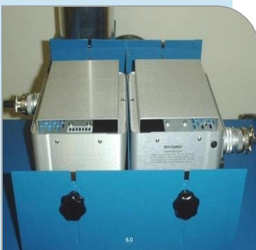
6. Install up to four reflector assemblies into the conveyor's upper lamp support brackets (2 shown above). Adjust the position of the lamps and tighten the four securing knobs.
