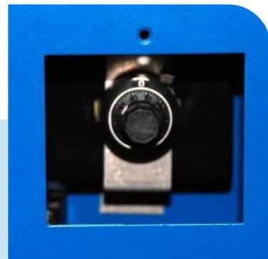
9. When the conveyor is operating, and the belt is in motion, turn each power supply on. Allow 5 minutes for the bulbs to reach full output intensity. If the temperature of the 5000 lamps are not around 122°F, remove the blower speed control cover and adjust the blower control knob to optimize bulb temperature. Wait about 5 minutes in between adjustments for temperature stabilization. Your UVCS Conveyor is ready for operation.
