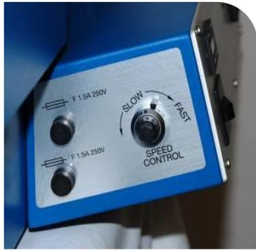
8. Turn the conveyor on by means of the power switch. Adjust belt speed by turning the speed control knob. Belt speed will be indicated on the speed display indicator.
