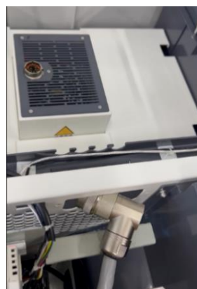
Figure 24 Cable Connector goes through the Wire Slot
