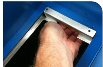
Figure 3. Install Frame Tab Above the Cradle Lip
