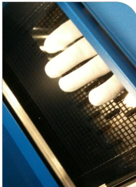
Figure 6. Position Quartz Window on Flange
