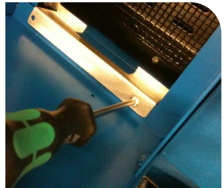
Figure 2. Installing Frame Tab
