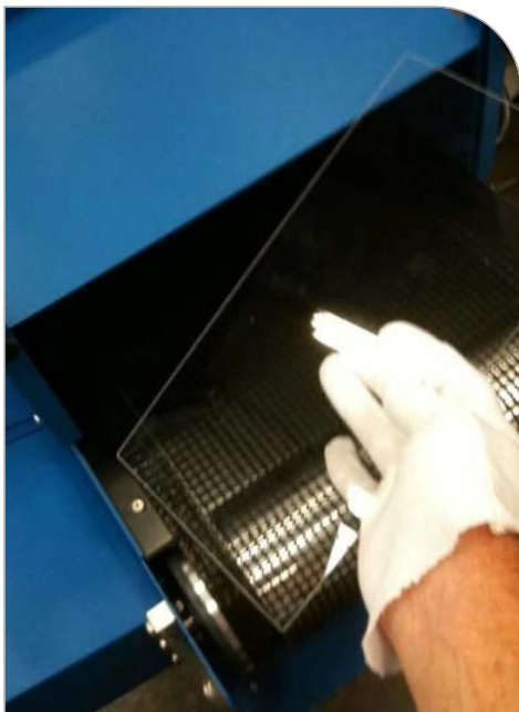
Figure 5. Installing Quartz Window in Conveyor
