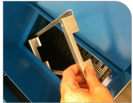
Figure 1. Installing Frames through Cradle Opening
