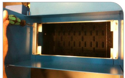
Figure 4. Installing Second Frame Tab
