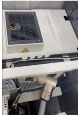
Figure 24. Cable Connector goes through the Wire Slot
