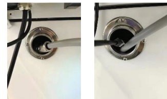
Install Connector and Network Wire on the Controller Connection
