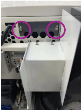
Figure 23. Loosen the Screws, remove the Wire Pressing Plate
