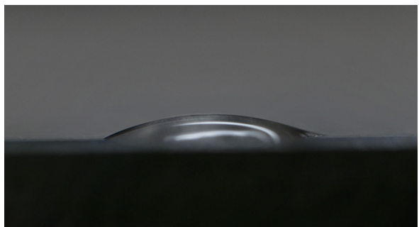
Figure 4. High-energy surface (liquid spreads out, indicating good adhesion)
