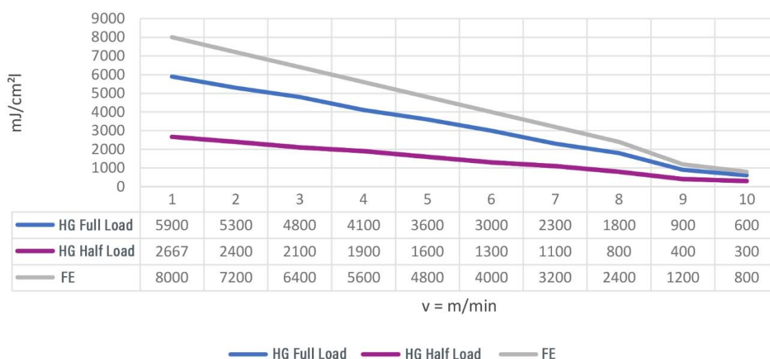
Figure 13. UV dose depending on the transport speed (1-10 m/min)
