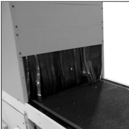
Figure 9. Conveyor Curing Chamber Entrance
