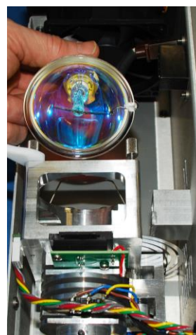
Figure 14. Remove Bulb from Bulb Mount
