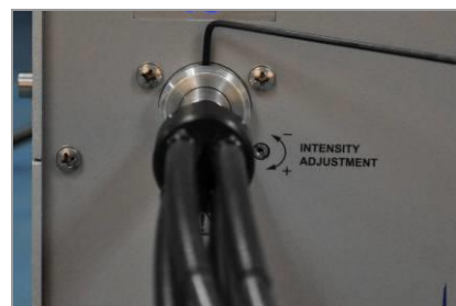
Figure 6. Tighten Setscrew on Lightguide Mount with Hex Wrench
