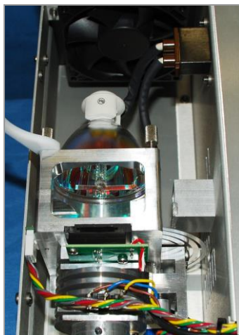
Figure 13. Lift Bulb Mounting Bracket
