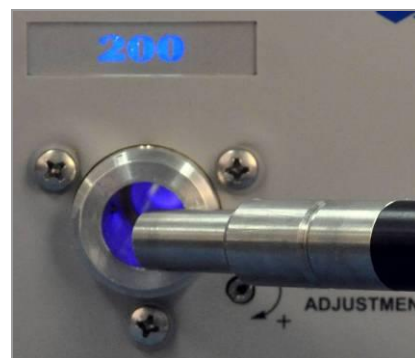
Figure 5. Insert Lightguide into Lightguide Mount
