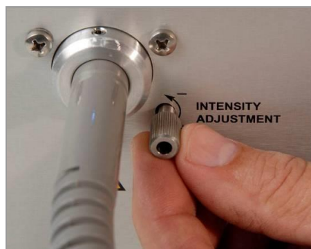
Figure 8. Intensity Adjustment with Knob
