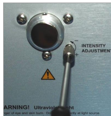
Figure 25. Intensity Adjustment Knob
