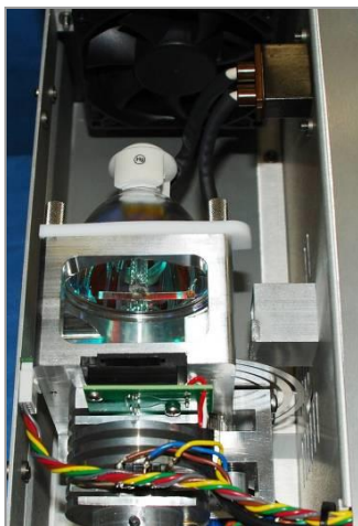
Figure 12. Bulb Installed in Bulb Mount
