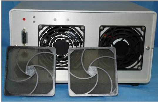
Figure 28. Exhaust Fans with Fan Filters Removed
