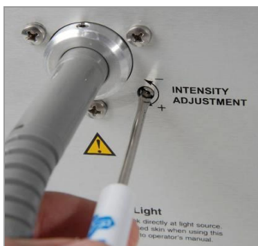
Figure 7. Intensity Adjustment with Tool
