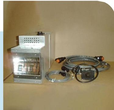
1. Uncrate the Conveyor and remove protective coverings. Place the conveyor on a convenient work surface. Install the exhaust ventilation stack on the blower motor's outlet flange. Secure the exhaust stack with the fasteners provided.
