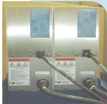
6. Attach the cables leading from the lamp(s) to the power supply(ies). Connect the conveyor's cable connector plugs into the J-105A, J-105B and J-106 receptacles. Connect each power supply's power cord to a 220 volt AC power source.
