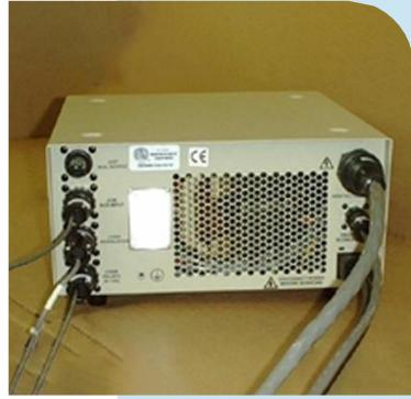
7. Plug the conveyor in to a 220 volt AC power source. Turn to conveyor on by means of the power switch. Adjust belt speed by turning the speed control knob. Belt speed will be indicated on the speed display indicator.
