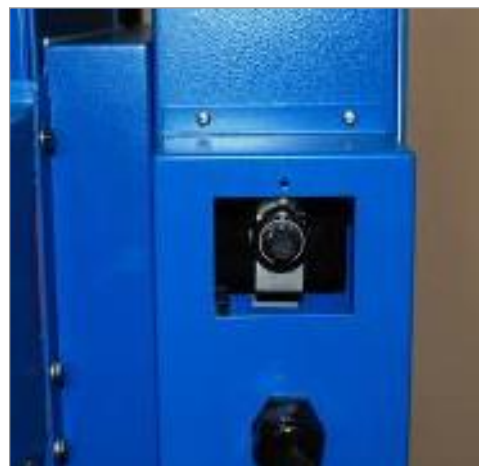
Figure 8. Blower Speed Control
