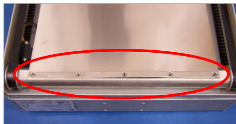
Figure 27. Five Retaining Screws
