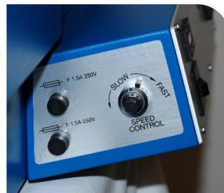
Figure 28. Conveyor Control Panel, Side
