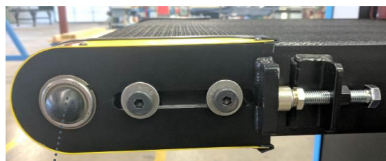
Figure 17. Adjustment Screws for Belt Tension and Alignment
