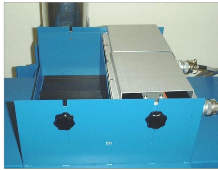
Figure 3. 5000-EC Mounted Side-by-Side on Conveyor
