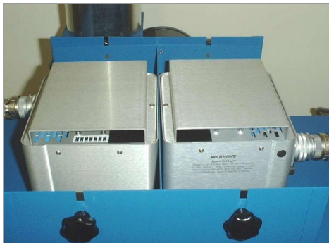
Figure 2. 2000-EC Mounted Side-by-Side on Conveyor
