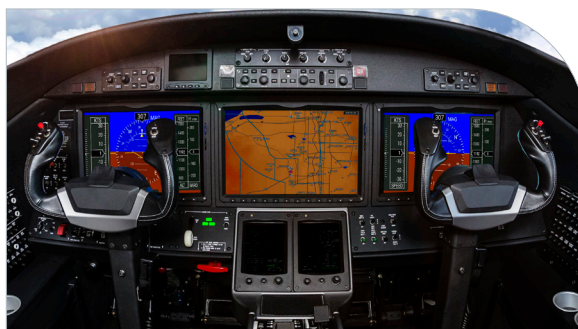
Optical bonding increases clarity, viewing angle, and vibration resistance
