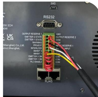
Controller PLC Socket
