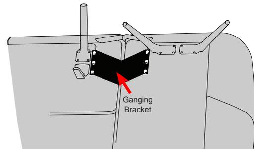
Under side view of the ganging bracket placement
