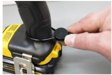
If the tether was removed, insert it back into the cable clamp. Slide the cable clamp up the tether so that it is tight against the merchandise.
