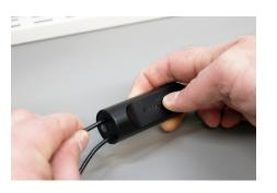
Plug the tether back into the housing.
