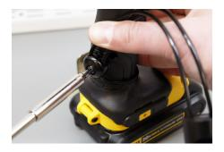
Tighten the screw using a TT20 bit.
