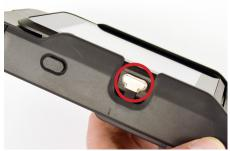
Plug the USB-C connector into the side of the payment device.
