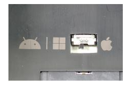
For CT3150 Only: Use the switch to select the type of tablet or handheld you are connecting to the E355: Android/ Windows or Apple.
