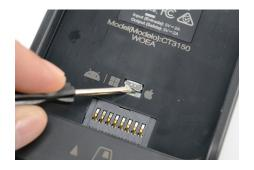
Use the small screwdriver to postion the switches to the appropriate settings.
